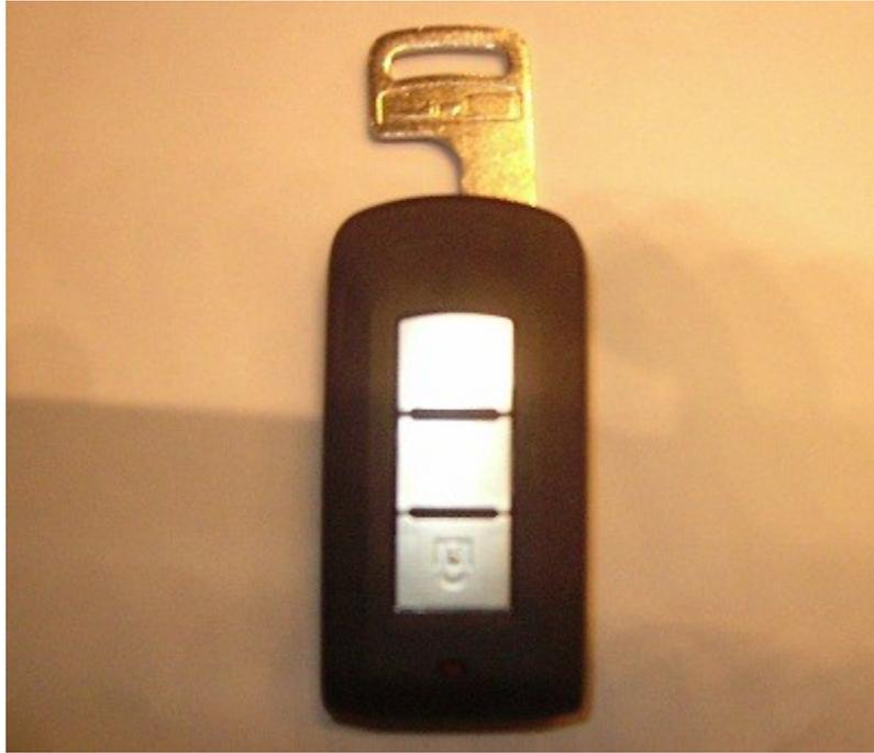
You must have a blade that will fit into the ignition lock of the vehicle.
