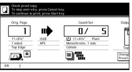
**5** After printing a single test copy, a confirmation screen will be displayed, and the copier will remain in standby mode until the job is approved or cancelled. Check the proof copy.
