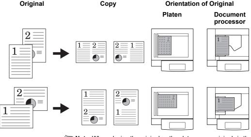
**Note** When placing the original on the platen, copy originals in the page order.
