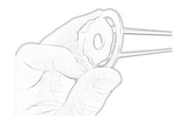
2. Fit gasket into circular groove on Conflat.
