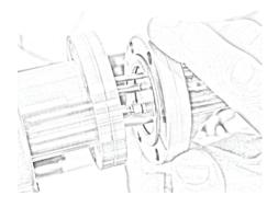
4. Press sensor head and feedthrough flanges together. Align bolt holes. Apply bolts and plate-nuts. Tightening bolts compresses copper gasket between a sharp edge and a tapered groove, thus creating a strong seal.
