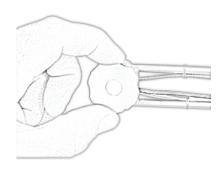
2. Flip cap over to access crystal retainer ring. Turn retainer ring COUNTER CLOCKWISE until loose.
