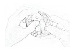
3. Flip crystal carousel and allow crystal to drop into sensor cap housing.
