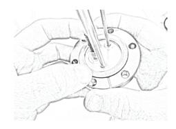
Hold copper gasket in place while inserting sensor head into chamber feedthrough.
