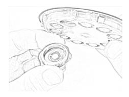
4. Use a plastic prod to adjust crystal position until crystal rests snugly in the crystal seat.
