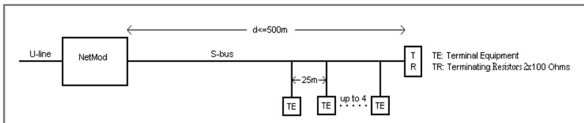
**Fig. 9: Extended passive bus connection**
