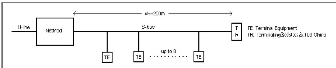
**Fig. 7: Short passive bus 1 connection**
