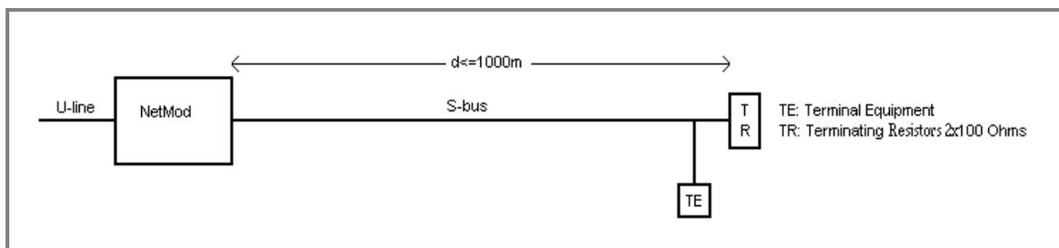
**Fig. 10: Point-to-point connection**
