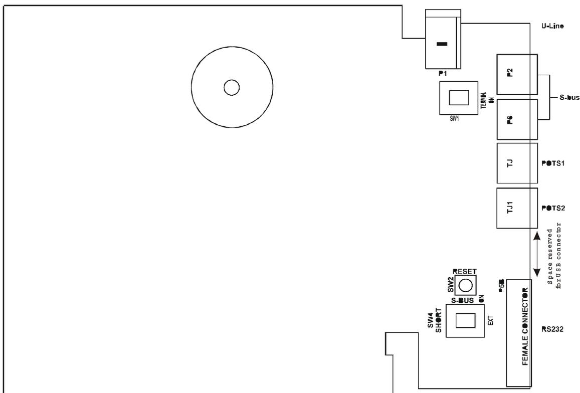
**Fig. 11: PCB layout of the motherboard (netMod) card**
