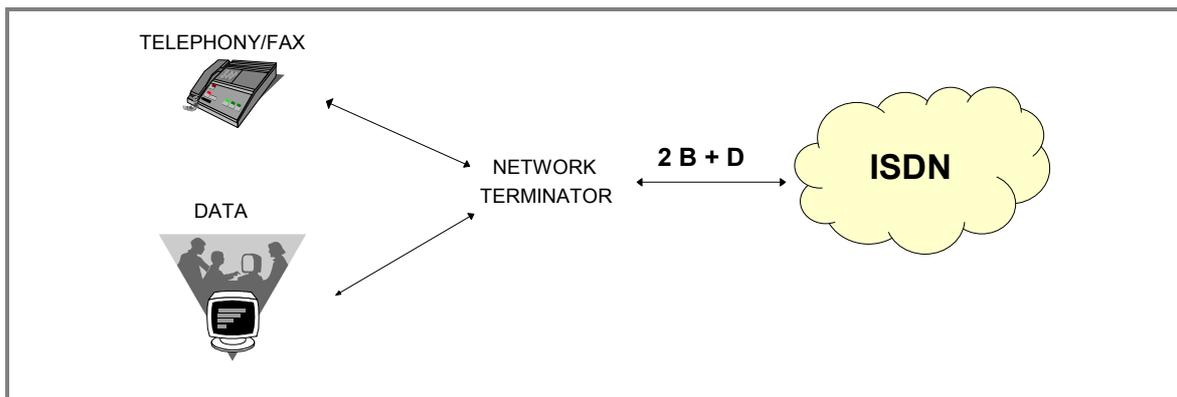
**Fig. 1: The basic access connection (BRA) between user and ISDN network**
