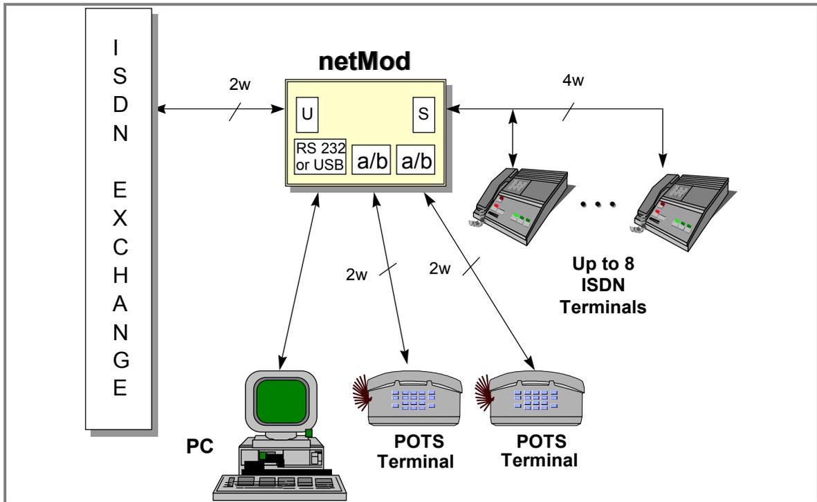
Fig. 4: netMod's connection with the subscriber's terminals (POTS, ISDN and PC) and the ISDN exchange
