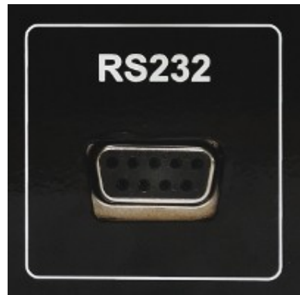
Fig. 10: RS232 controller connector
