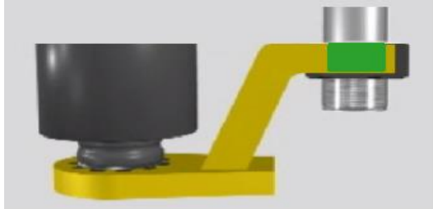
Figure 4.1.4-1: Correct Reaction Point
