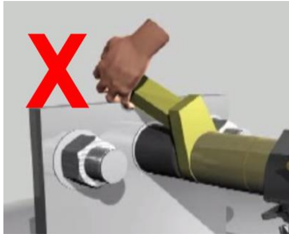
Figure 4.1.1-2: Incorrect Placement of Hand/Body Parts During Operation
