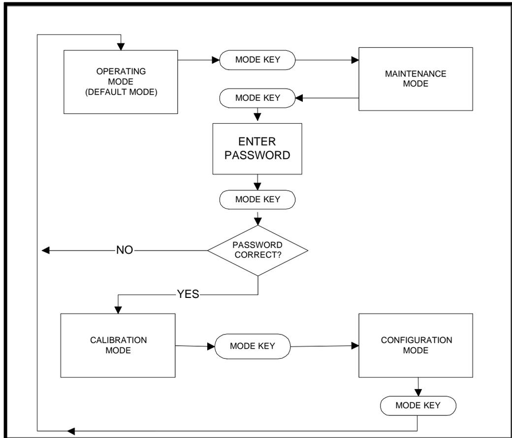
To enter the CONFIGURATION mode from the OPERATING mode, press the **MODE** key twice. The next screen prompts for the password. Use the **CLEAR** and **PRINT** keys to enter the password. Press the **MODE** key to enter the CALIBRATION mode. Press the **MODE** key again to gain access to the CONFIGURATION mode. If the CONFIGURATION mode is reentered, assuming no power loss, the unit displays the last CONFIGURATION field selected.
