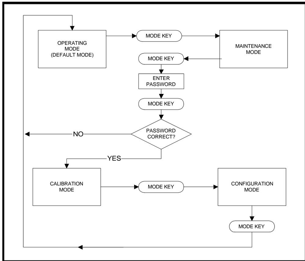
The OPERATING mode is the normal or default mode of operation of the ACE. If the unit is in the MAINTENANCE mode, press the **MODE** key twice to place the ACE into the OPERATING mode. If the unit is in the CALIBRATION mode, press the **MODE** key twice, or if in CONFIGURATION mode press the **MODE** key to return the ACE to the OPERATING mode.
