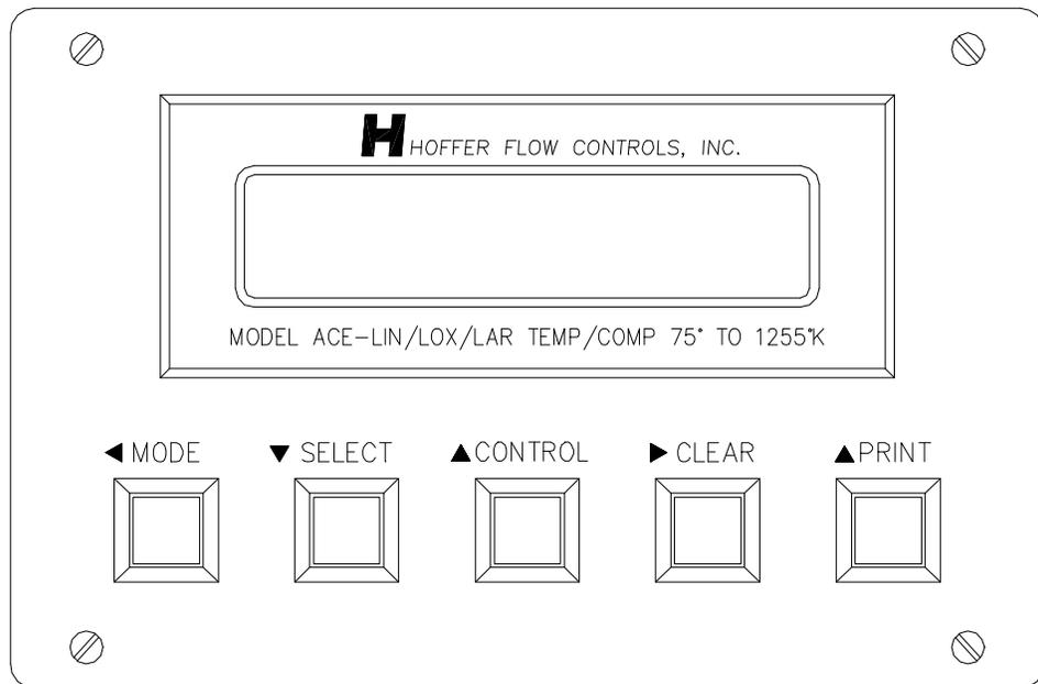
Program control keys consist of the **MODE** (left arrow), **SELECT** (down arrow), **CLEAR** (right arrow), **PRINT** (up arrow), and **CONTROL** key.
