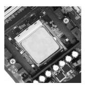
2. If required, apply a light coating of silica gel to the top of the CPU.
