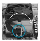
5. Push down the retention bracket lock on the retention mechanism to secure the heatsink and fan to module base.
