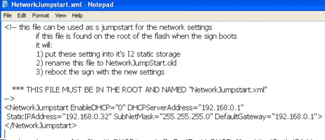
The above is a copy of the file with DHCP turned off. Ex. "EnableDHCP=0" and the "Static IPAddress" specified along with the "SubNetMask" and "DefaultGateway".
