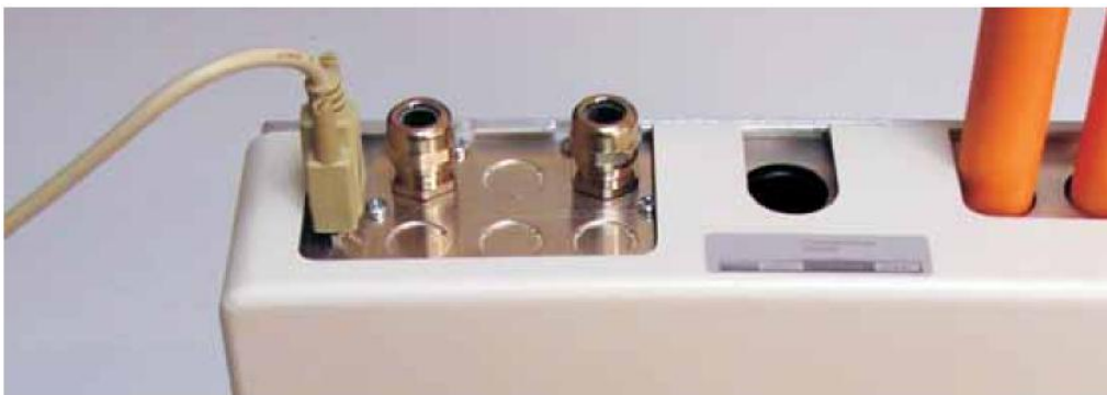
Figure 25: Connecting a PC to the command module's RS-232 port
