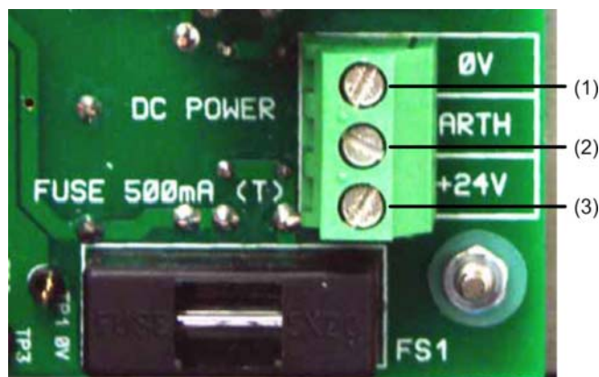
Figure 18: Command module power supply connections
