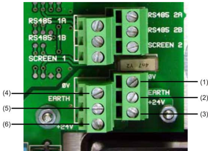
Figure 17: Detector power supply connections
