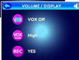
NOTE: **VOX** keeps monitor (picture and sound) off until the camera detects a sound, which automatically turns the monitor back on. This helps prevent false alarms and allows parents more rest.
