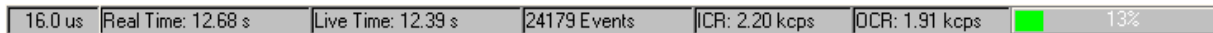
Figure 4: The run statistics bar in Kepler. This bar shows a summary of run statistics, updated automatically at the end of all runs and at the user defined update interval. The statistics can also be updated by pressing the [Refresh] button.
