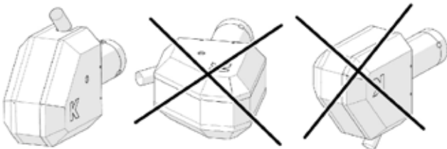
Fig.: Burner installation
