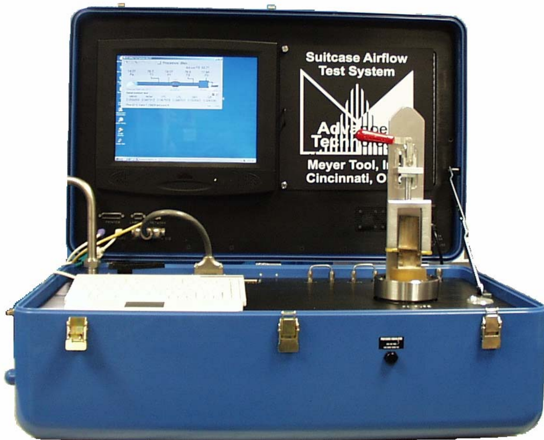
Figure One: 5000-33-3702NA5, Suitcase Airflow Test System, Cart Design
