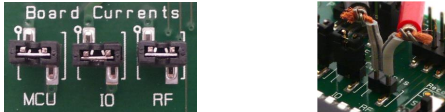
Figure 16 – Current measurement jumpers
