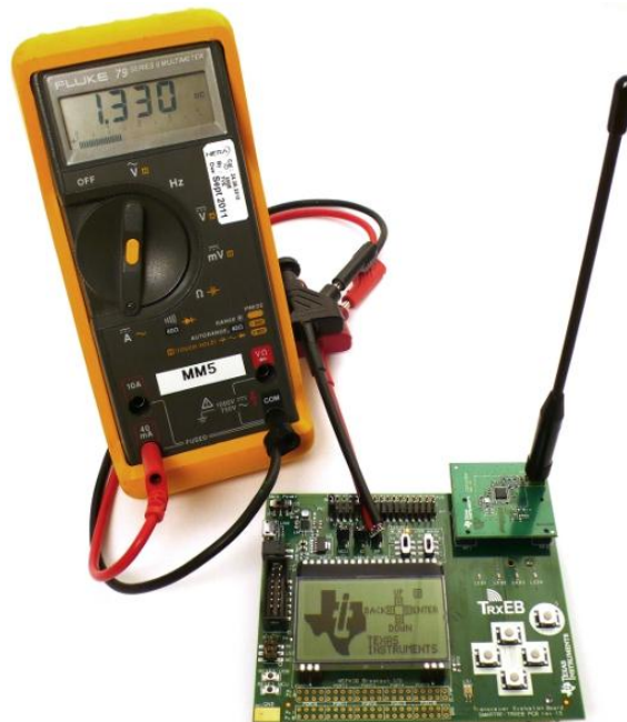
Figure 17 – Current measurement setup
