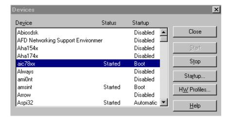
Ensure the aic78xx entry under Device displays 'Started' under Status and 'Boot' under Startup as seen here. Ensure 'Aspi32' entry under Device displays 'Started' under Status and 'Automatic' under Startup as seen above.
