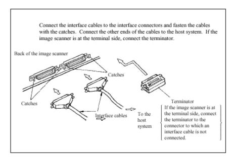
Typically the SCSI ports are located on the back of the scanner (the one exception being the Fi-5650C which is on the front). Depending on the model the SCSI port connector(s) may be any one of the following:
