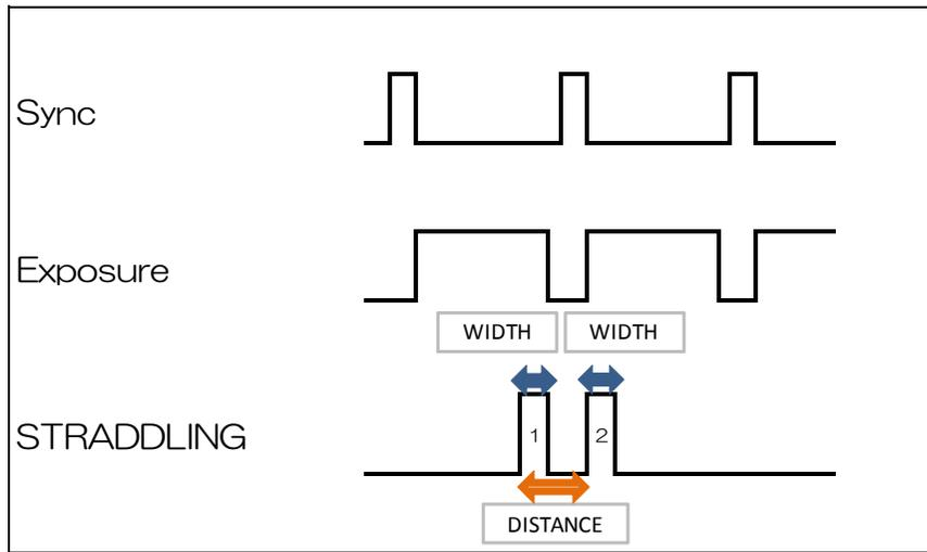
While the minimum width is fixed to 100 ns, the minimum distance is variable depending on shutter speed.
