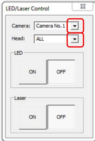
7. Make a necessary setting of ON or OFF for LED and Laser, respectively.
