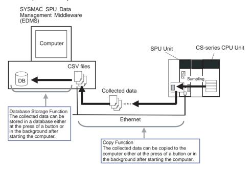
Save copied files to any folder on the computer (see note) and automatically create file names using any combination of objects, i.e., any text string, time, or consecutive file numbers.
