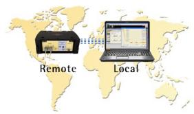
Software upgrades via USB memory or LAN (through STT Controller or PC)
