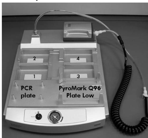
**Figure 23. Placement of PCR plate (or strips) and PyroMark Q96 Plate Low or PyroMark Q96 HS Plate on the PyroMark Q96 Vacuum Workstation.** The marked positions contain 70% ethanol (1), PyroMark Denaturation Solution (2), PyroMark Wash Buffer (3), and high-purity water (4).
