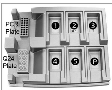
**Figure 9. Placement of PCR plate and PyroMark Q24 Plate on the PyroMark Q24 Vacuum Workstation.** The marked positions contain 70% ethanol (1), PyroMark Denaturation Solution (2), PyroMark Wash Buffer (3), and high-purity water (4, 5). P: Parking position.
