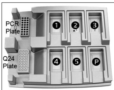
Figure 22. Positions on the PyroMark Q24 Vacuum Workstation.
