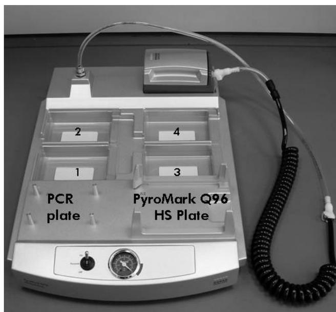
**Figure 19. Placement of PCR plate (or strips) and PyroMark Q96 HS Plate on the PyroMark Q96 Vacuum Workstation.** The marked positions contain 70% ethanol (1), PyroMark Denaturation Solution (2), PyroMark Wash Buffer (3), and high-purity water (4).
