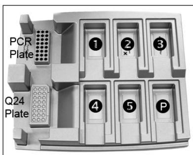
**Figure 5. Placement of PCR plate (or strips) and PyroMark Q24 Plate on the PyroMark Q24 Vacuum Workstation.** The marked positions contain 70% ethanol (1), PyroMark Denaturation Solution (2), PyroMark Wash Buffer (3), and high-purity water (4, 5). P: Parking position.
