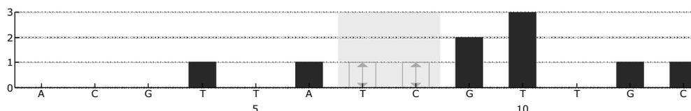
**Figure 4. Histogram for AQ mode.** Nucleotide additions 1, 2, 3, 5, and 11 are blank and serve as negative controls. The seventh and the eight dispensations analyze the variable position.
