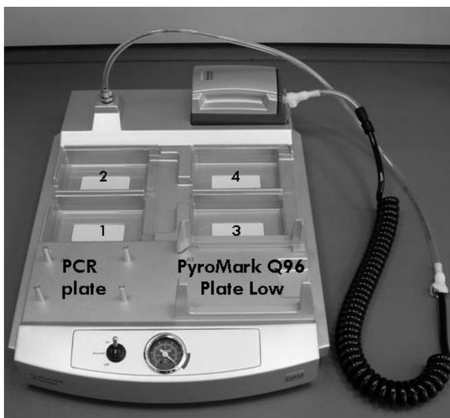
**Figure 14. Placement of PCR plate (or strips) and PyroMark Q96 Plate Low on the PyroMark Q96 Vacuum Workstation.** The marked positions contain 70% ethanol (1), PyroMark Denaturation Solution (2), PyroMark Wash Buffer (3), and high-purity water (4).
