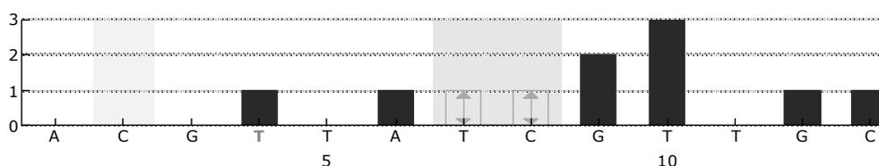
**Figure 18. Histogram from PyroMark CpG Software.** Nucleotide additions 1, 2, 3, 5 and 11 are blank dispensations and serve as negative controls. The seventh and the eighth dispensations analyze the variable position (wobbled/degenerated base).
