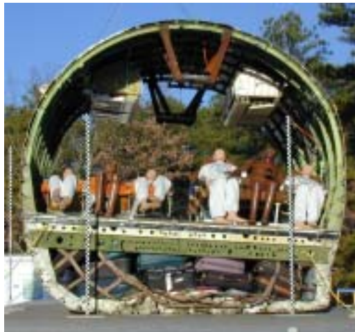
Figure B-2. Post-test photograph of the B737 fuselage section with bins and luggage.
