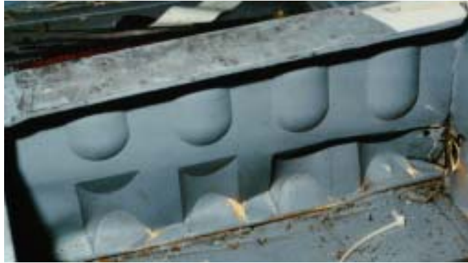
(a) Photograph of the subfloor consisting of two horizontal C-channels, one above the other with a beaded (or waffle) web geometry.
