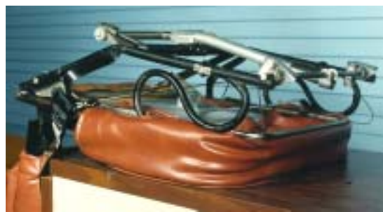
Fig. 10. Deformed JAARS seats, post-test.
