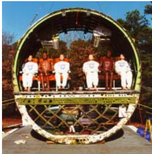
Figure B-1. Pre-test photograph of the B727 fuselage section with overhead bins and luggage.
