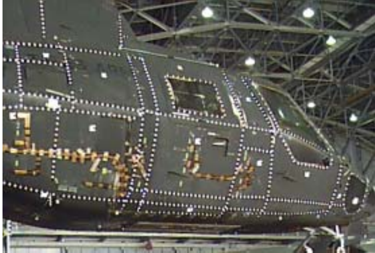
Figure A-5. Photograph of the ACAP helicopter during the photogrammetric survey.
