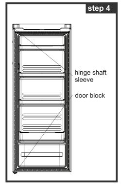
5. Take the hinge and undo the nut holding the hinge pin. Relocate to the opposite side and fix in place.
