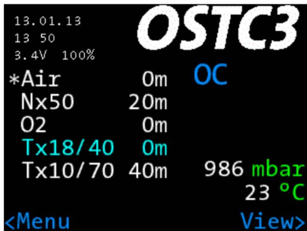
When in surface mode, the display shows general information – current time, date, temperature, ambient pressure and battery status. After a dive, the display also shows tissue saturation and remaining time in the no-fly period. In surface mode, you can adjust the settings in preparation for the next dive, read recorded dive data and adjust the base settings of the OSTC3
