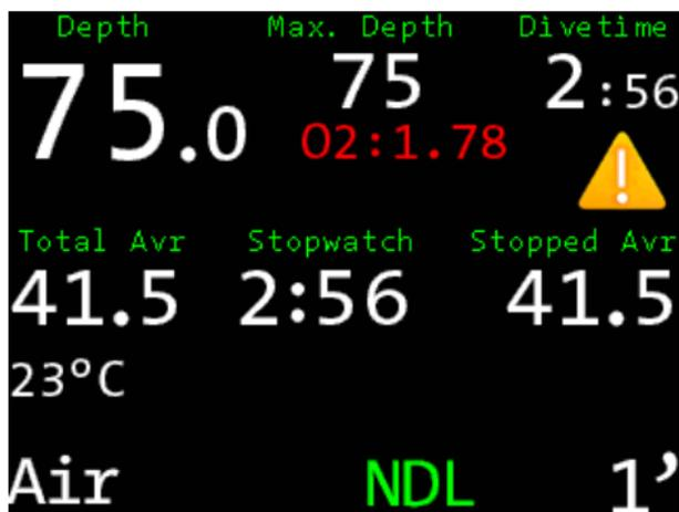
The OSTC3 automatically switches into dive mode when it is at least 1.6 m below the surface for five seconds.
