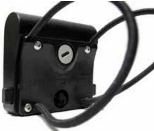
OSTC3 is shipped with bungees. The bungees can be detached, are hand washable and can be replaced if necessary. In order to replace the bungee remove the four screws (2mm Allen key) and detach the lower housing plate. Align the new bungee in a loop around the USB-bulkhead and put the ends through the two holes in the lower housing plate. Only use the screws supplied with OSTC3. They are non-corrosive and that is very important in that case.
