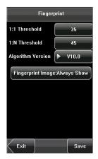
fingerprint and the fingerprint template enrolled in the Device is larger than this threshold, the matching is successful; otherwise, the matching is not successful.
