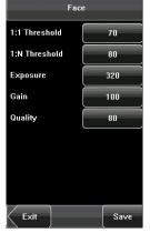
**1:1: N Threshold:** This parameter is used to set the threshold of matching between current face and the face
