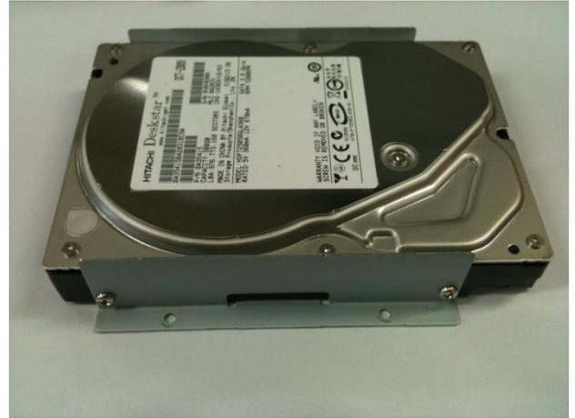
2. The mounted HDD(DVDRW) with the mounting brackets.
