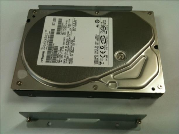
1. Before installing, mounting brackets and screws onto HDD(DVDRW).
