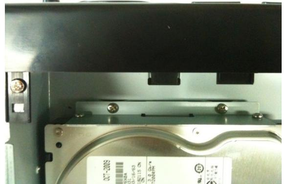
4. Install HDD(DVDRW) with fixing screws onto the inside of the system
