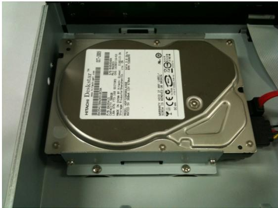
3. Install HDD(DVDRW) with fixing screws onto the inside of the system
