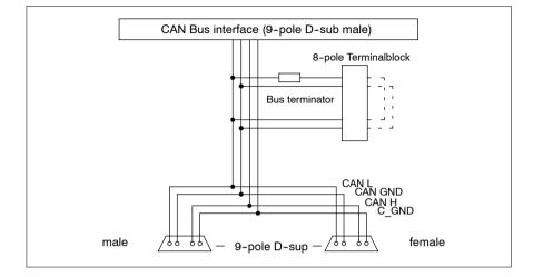
Figure 53 Function of the CAN-TAP
