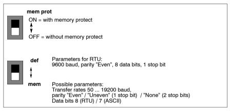
The memory protect switch "mem prot" prevents modifications to the user program with a programming device (ON).
