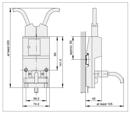
Figure 39 470 NAV 511 dimension drawing (units in mm)
