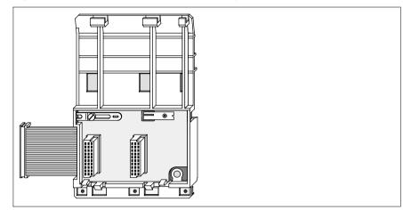
Figure 61 Front view of the AS-HDTA-202 backplane
