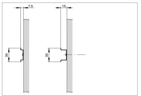
Figure 19 Top hat rail with 7.5 mm clearance (left) and with 15 mm clearance (right)
