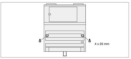
The screws are used to ground the module.
