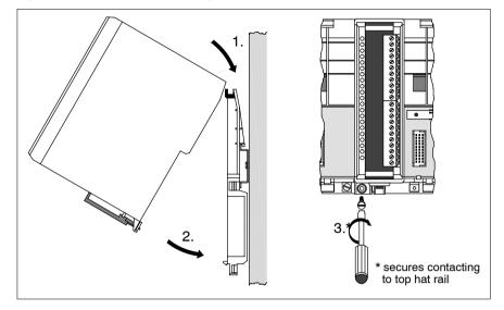
Figure 25 Installation of remaining modules
