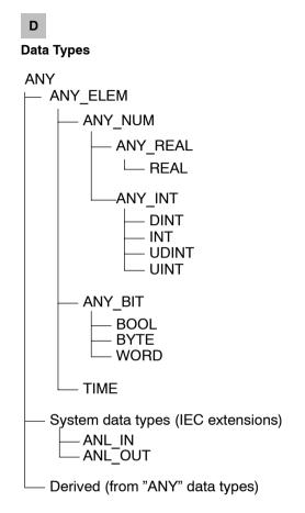
The overview shows the hierarchy of generic data types as they are used by the inputs and outputs of functions and function blocks. Generic data types are identified by the prefix "ANY".
