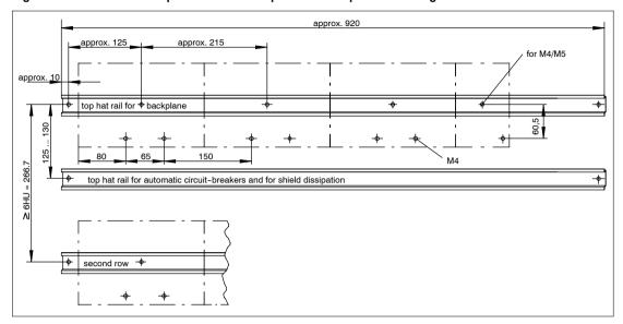
Figure 20 Drill holes for top hat rail and backplane in back panel mounting
