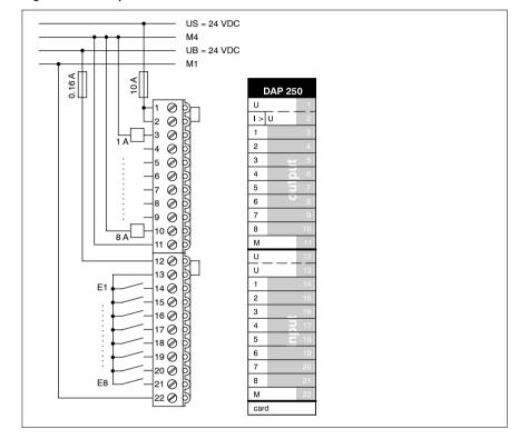
Figure 43 Example of connection
