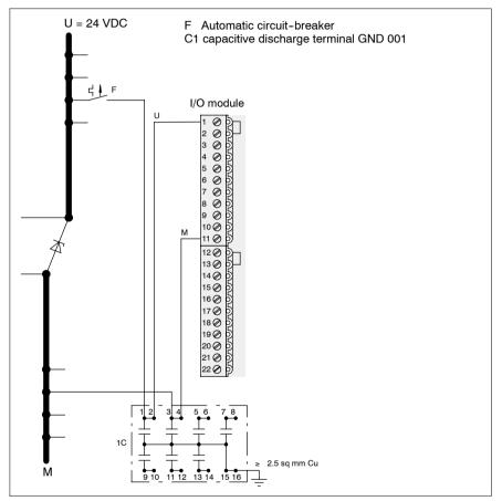
In an interference-prone environment, it is recommended to increase the capacity on the C1 from 2.2 nF to 22 nF.
