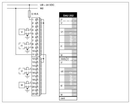
Figure 49 Example of connection
