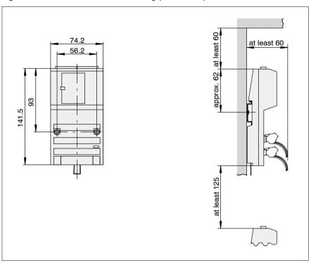
Figure 38 470 IPS 258 dimension drawing (units in mm)
