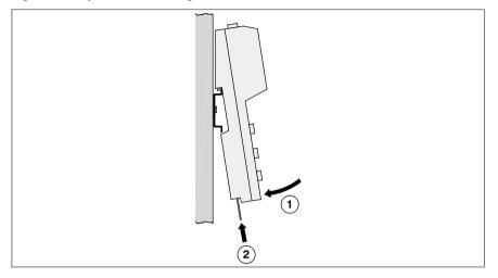
The grounding spring integrated into the right back panel establishes the electric contact to the top hat rail.
