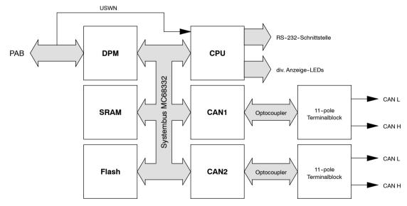
Motorola Processor 68332-16 (16 MHz) 64 K/ 16 Bit SRAM, 64 K/ 16 Bit FLASH, 8 K Byte DPM
