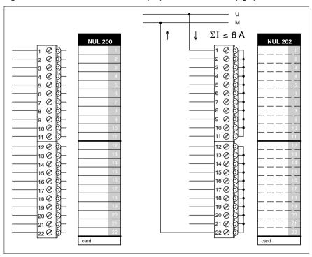
Figure 58 Connections AS-BNUL-200 (left) and AS-BNUL-202 (right)
