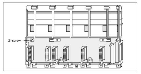
Figure 59 Front view of the AS-HDTA-200 backplane
