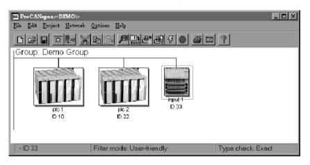
If the ASBC259.EDS file of AS-BCAN-259 is located in the ProCanopen \EDS subdirectory and the module is configured by the CIA\_SVR EFB (see chapter CIA\_SVR) the module will be recognized by ProCANopen.
