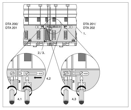
Figure 23 Coupling DTA 200 or DTA 201 with DTA 201 or DTA 202
