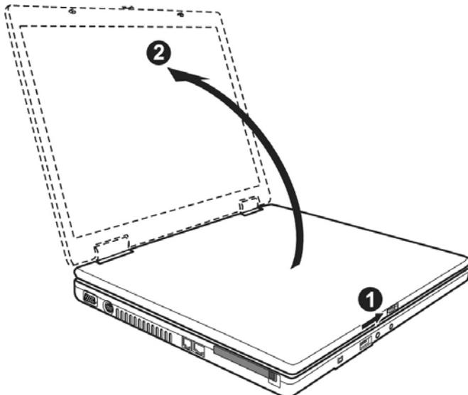
To open, use your thumbs to push the bar to the right (1) then lift (2) the display with your thumbs and index finger and position it as desired.
