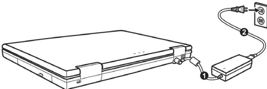
The adapter provides the notebook with power and also charges the battery. The power supply indicators of the notebook provide details on the operating state. The battery is also being charged when you are working on your notebook with the power adapter. The power adapter is still live if the notebook is not connected with it. You should therefore unplug the power adapter from the outlet if it is not connected to the notebook.
