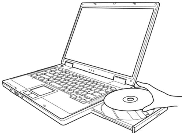
5. Test that the disk is able to turn freely and then push the tray back into the optical drive carefully.
