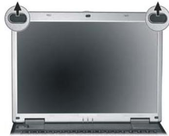
4. Remove the screws on both sides.
