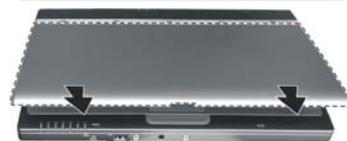
6. Replace the clip-on cover with a new one by aligning the five notched hole.
