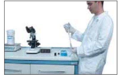
Concentration analysis with Medi Chimica digital colorimeter SPERMDENS.
