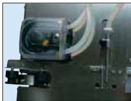
High flow rate peristaltic pump for a lower stress of the seminal material
