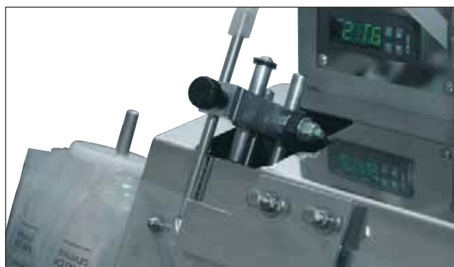
Electronic check of weld temperature, filling timer and AUTO switch
