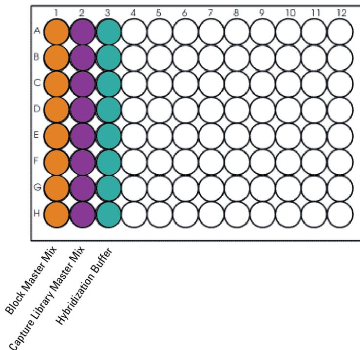
**Figure 11** Configuration of the master mix source plate for Hybridization\_MMCol\_v2.0.pro. Each well in column 2 may contain the same or different Capture Libraries.
