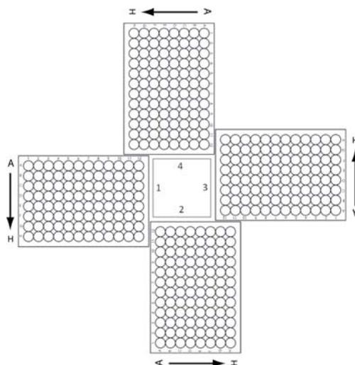
**Figure 6** Labware MiniHub plate orientation. For Thermo Scientific reservoirs, place the notched corner facing the center of the hub.
