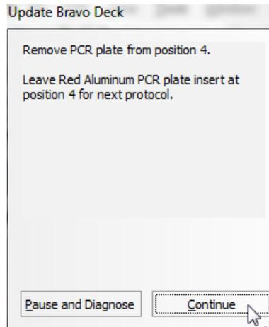
The remainder of the SureSelectCapture&Wash\_v2.0.rst runset takes approximately 1.5 hours. Once the runset is complete, the captured, bead-bound DNA samples are located in the Eppendorf plate at position 9 of the Bravo deck.
