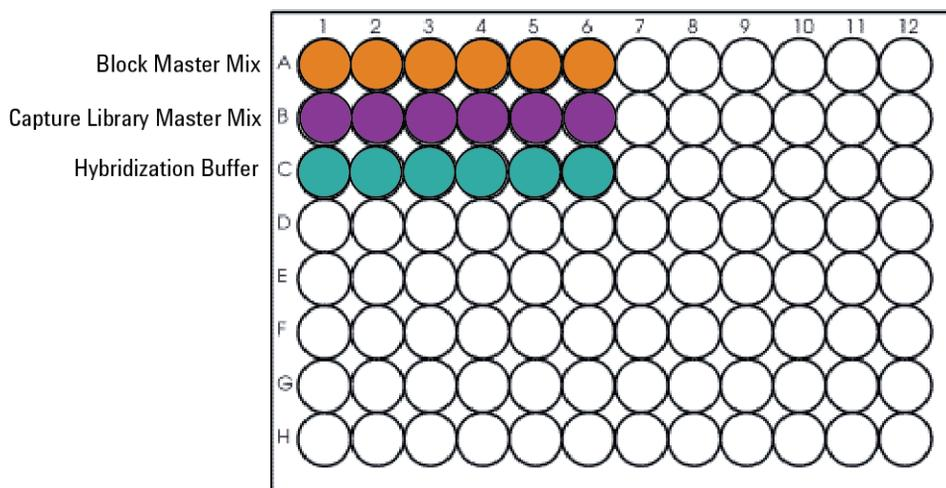
**Figure 12** Configuration of the master mix source plate for Hybridization\_MMRow\_v2.0.pro. Rows A–C may contain 1, 2, 3, 4, 6, or 12 wells of reagents, depending on run size (example shown is for 6-column run size). Each well in row B may contain the same or different Capture Libraries.
