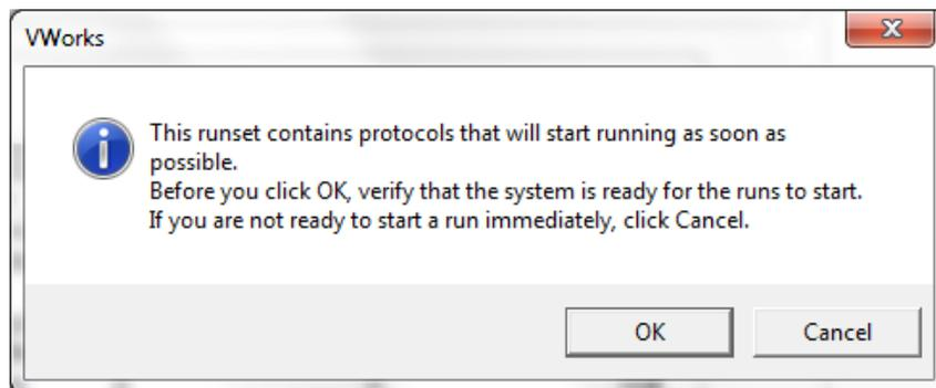
Running the LibraryPrep\_XT\_Illumina\_v2.0.rst runset takes approximately 3 hours. Once complete, the purified, indexing adaptor-ligated DNA samples are located in the Eppendorf twin.tec plate at position 7 of the Bravo deck.
