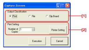
The capture function screen can be displayed by pressing "Capture" button at the bottom of each screen.
