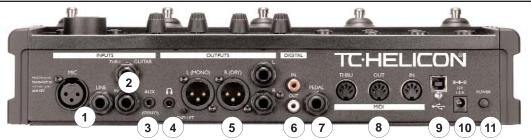
I. MIC and LINE inputs - Connect your microphone or line level audio device's output here. Only one should be connected at a time. Hold the REVERB footswitch to set gain when changing back and forth between MIC and LINE ins.
