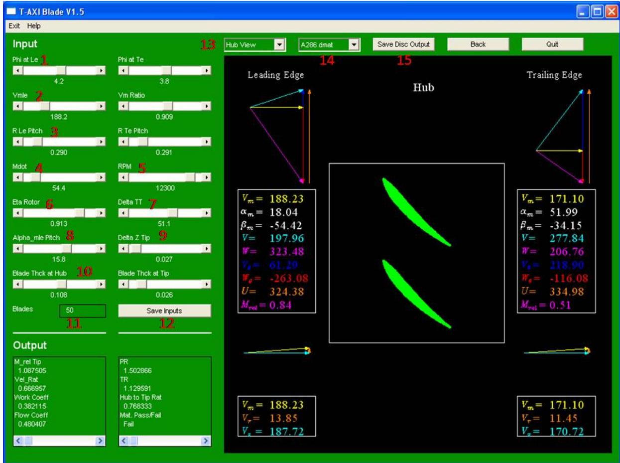
Figure 2: T-AXI Blade Main Window.
