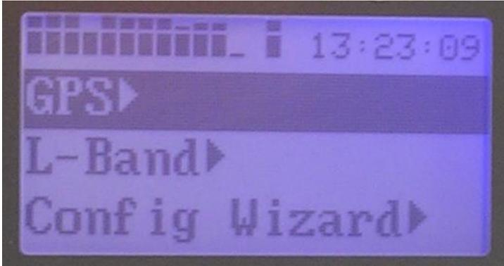
Figure 6: the receiver main screen
