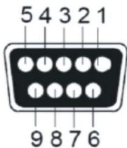
Figure 14 : DB9 pin layout on receiver (female connector)
