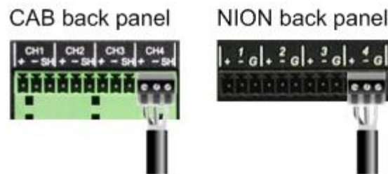
Analog balanced audio connection using standard cable
