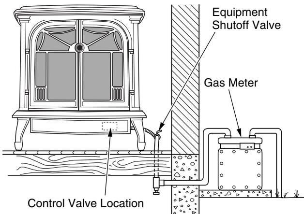
**Figure 11 - Checking Gas Joints on Natural Gas Unit**
