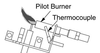
Figure 19 - Incorrect Pilot Flame Pattern (Propane/LP Shown)
