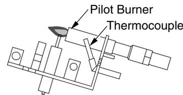
Figure 18 - Correct Pilot Flame Pattern (Propane/LP Shown)
