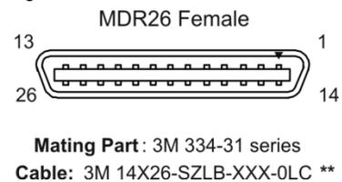
**\*\*3M part 14X26-SZLB-XXX-OLC is a complete cable assembly, including connectors. Unused pairs should be terminated in 100 ohms at both ends of the cable.**
