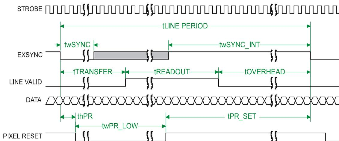
Figure 5: Piranha 3 Fixed (Programmed) Integration Timing with External EXSYNC
