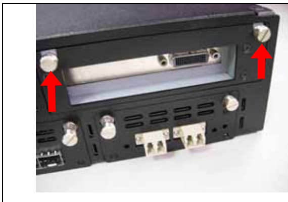
Fig. 2-11c Loosen the screws.
