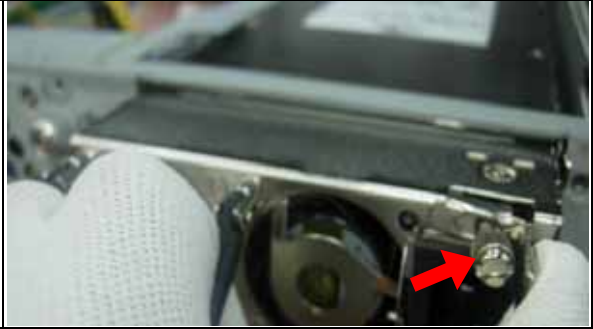
Fig.2-21.2 Pull out the power modules.
