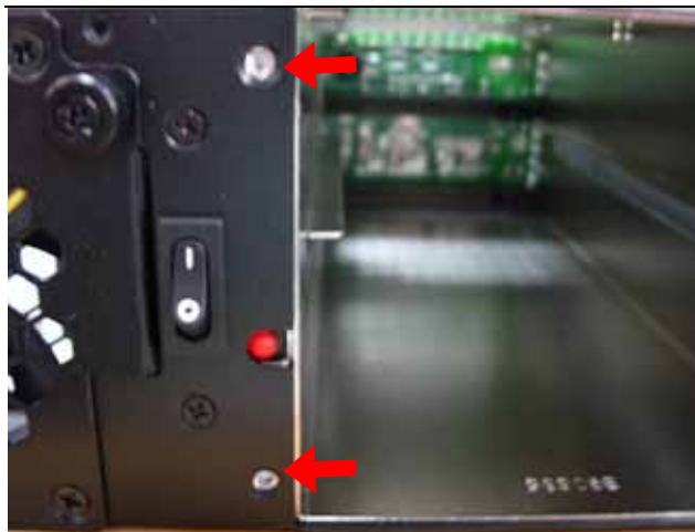
Fig.2-25.3 Remove the screws.
