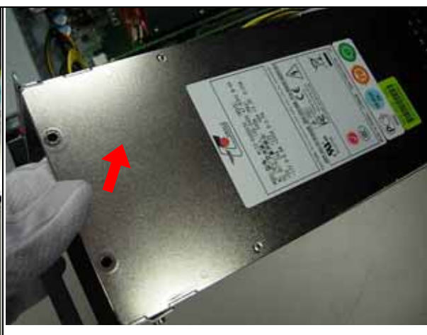
Fig.2-26.2 Lift up and Pull out the power supply.
