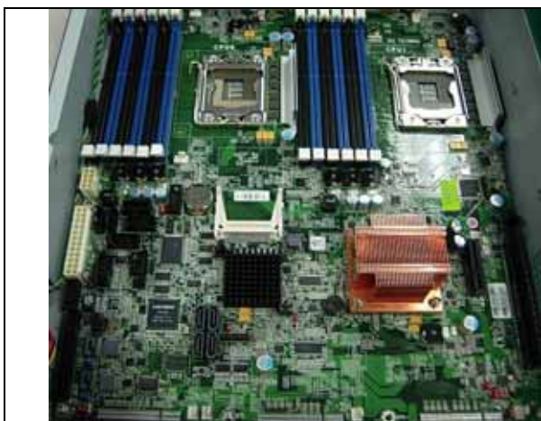
Fig.2-31 Remove all screws from main board.
