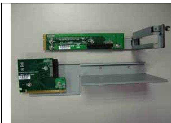
Fig. 2-11e Loosen the screws and remove riser.
