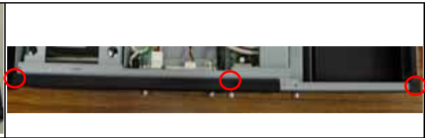
Fig.2-17b Remove screws and front panel.
