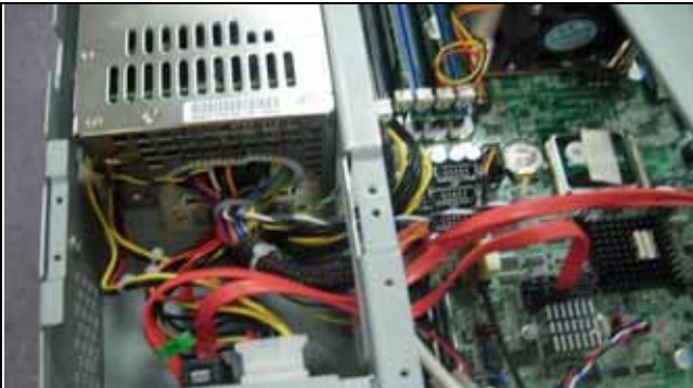
Fig.2-23 Remove all power cables from board and HDD bay.
