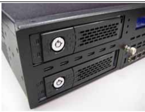
Fig. 2-12b Fix HDD into CAR-5010 system
