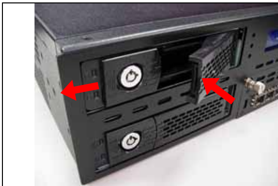
Fig. 2-12a Connect HDD bracket to CAR-5010 system then push the switch in.
