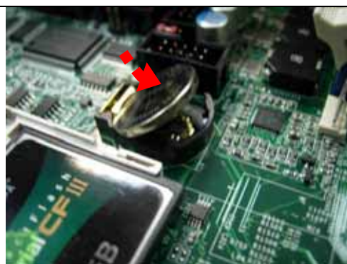
Fig. 2-10 Restore the battery
