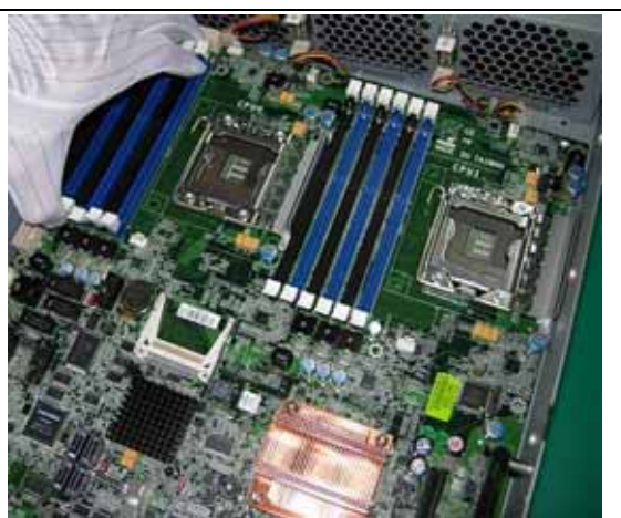
Fig.2-32 lift up main board from system from rear-left side.
