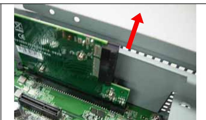
Fig. 2-11f Remove the riser card and bracket
