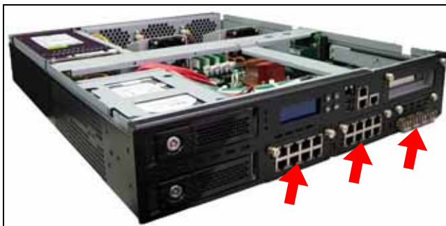
Fig.2-27 Remove all add-on modules.
