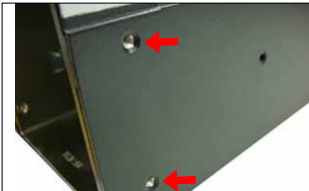
Fig.2-25.1 Remove the screws.
