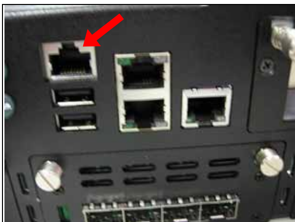
Fig.2-36 Connect null serial port cable to CAR-5010 console management port.
