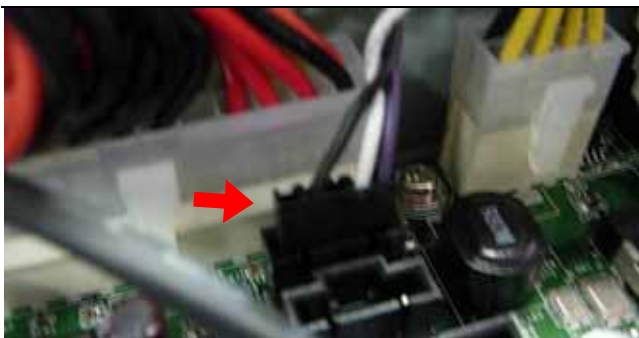
Fig.2-25 Remove I2C cable.
