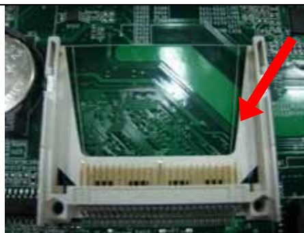
Fig. 2-7 Insert Compact Flash Card into the CF interface
