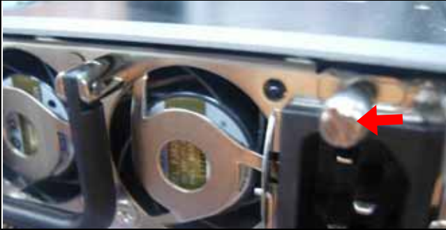
Fig.2-21.1 Loosen the screw to unlock the power module.
