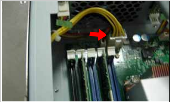
Fig.2-24 Remove all cables from the board.
