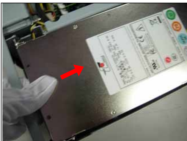
Fig.2-26.1 Push the power supply into system first.
