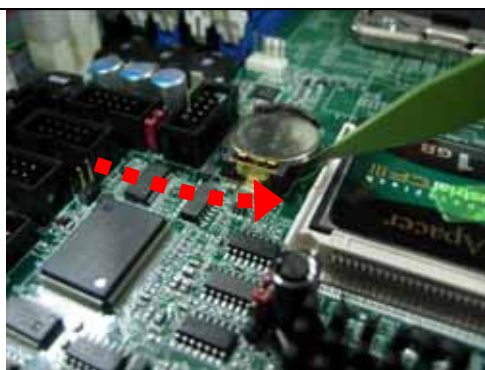
Fig. 2-9 Eject the battery
