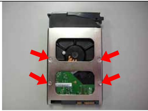
Fig. 2-11b Fix HDD to the bracket
