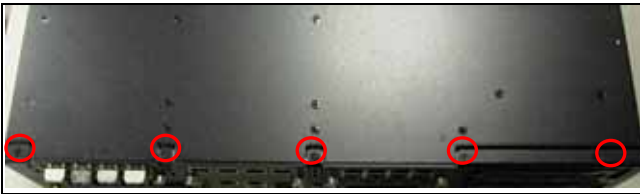
Fig.2-17a Remove front panel first. Remove 5 screws.
