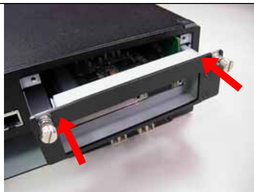
Fig. 2-11b Fix riser card/ add-on card to CAR-5010
