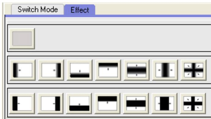
The device VSP 729 2U not only provides the most common fade effects( in default), but also other fourteen seamless transition effects: wipe right, wipe left,wipe up, wipe down, wipe center out, wipe curtain out, wipe square out, etc.
