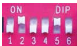
Block with 6 dipswitches
