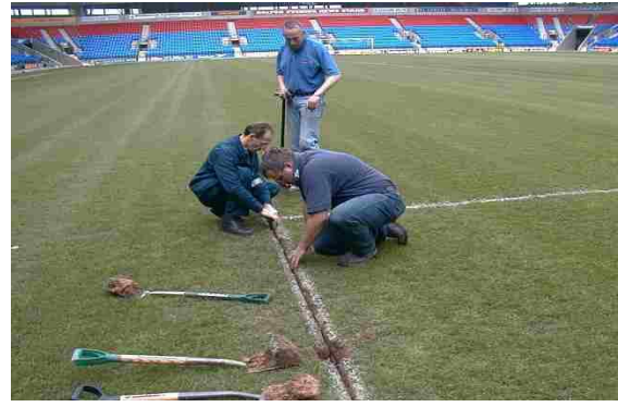
Push sensor to desired depth
