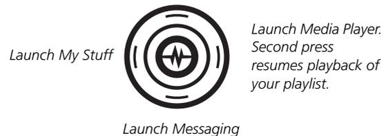
Your Amp'd Mobile™ Jet has a 5-way navigation key with a round, blue **Amp'd Live™** button at the center surrounded by a 4-way circular navigation key. The blue **Amp'd Live™** button has the following functions:
