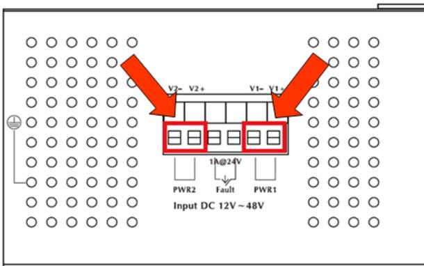
2. Tighten the wire-clamp screws for preventing the wires from loosing.
