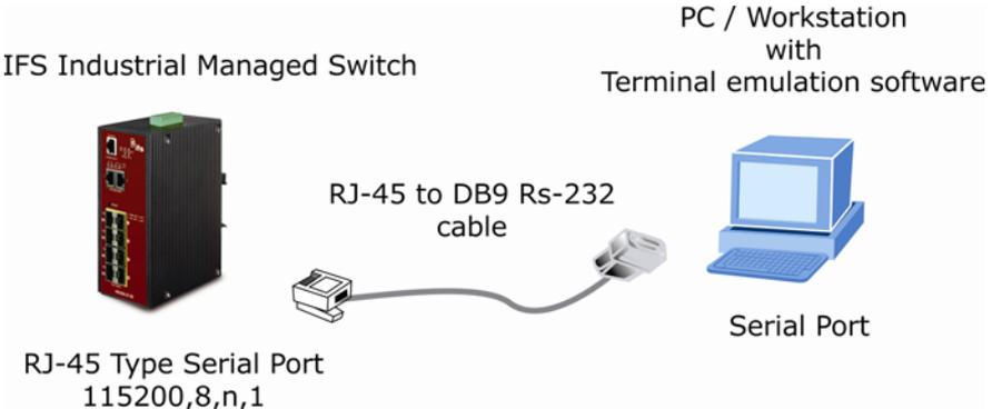
A terminal program is required to make the software connection to the IFS Managed Industrial Switch. Windows' **Hyper Terminal** program may be a good choice. The Hyper Terminal can be accessed from the **Start** menu.
