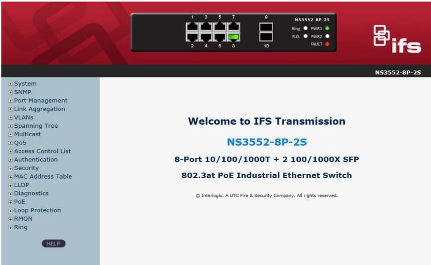
**Figure 7-3:** Web Main Screen of Industrial Managed Switch
