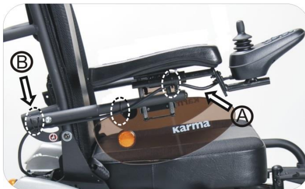
Controller Cable Tie Locations
