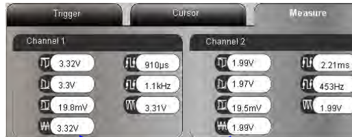
Figure 2-37: Resistor Voltage Measurements and Current Calculations ( HomeWork Board )
