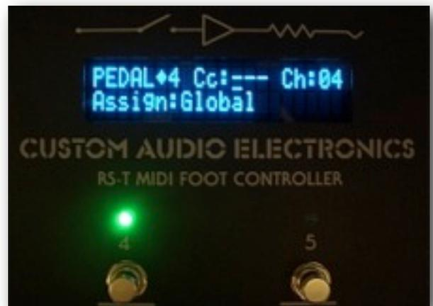
**Note: If you are assigning cc Pedal commands per Preset, start from the Bank/Preset you want to send from BEFORE entering the PEDALS page in Edit Mode**
