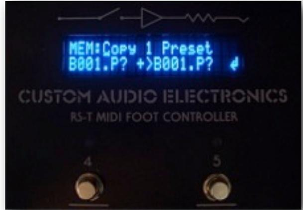
9. Once the operation is complete the display will return to the MEM page with the block cursor flashing over the carriage return symbol. You can now exit this page or Edit Mode by pressing ENTER/UNDO.
