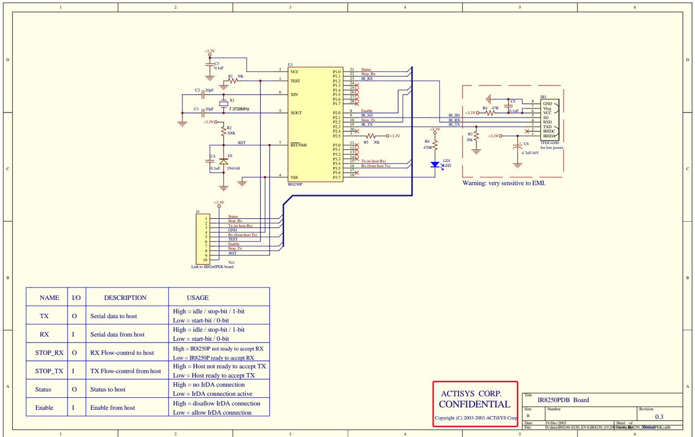
PCB footprint & dimensions, part number, supplier and pinout spec for the connector J1 on ACT-IR8250x0PMB and ACT-IR8250PDB boards are as follows: Molex, part number SD-48148. You can get dimensional information at: [www.molex.com](http://www.molex.com). More details on [section 5.1](#).
