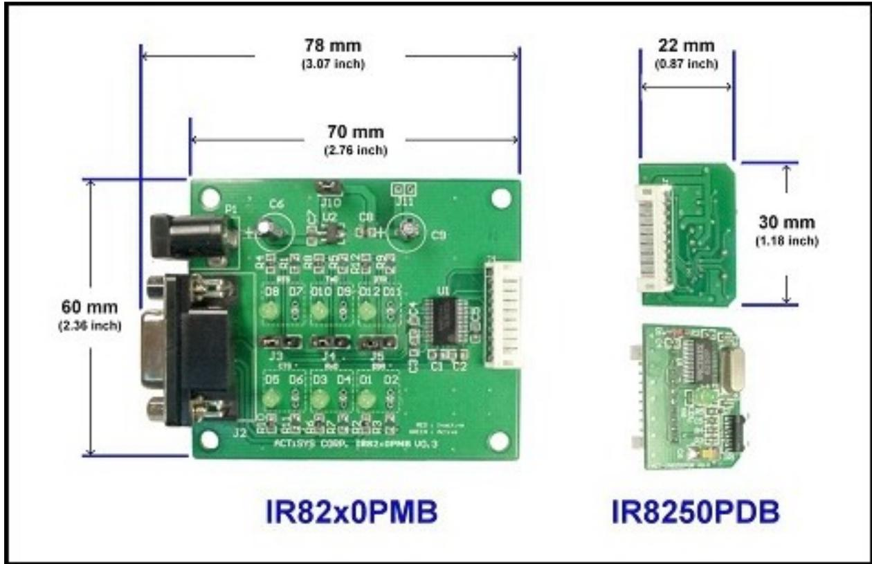
PCB footprint & dimensions, part number, supplier and pinout spec for the connector J1 on IR8250x0PMB and ACT-IR8250PDB boards are as follows: Molex, part number SD-48148. You can get dimensional information at: [www.molex.com](http://www.molex.com). More details on the next page.
