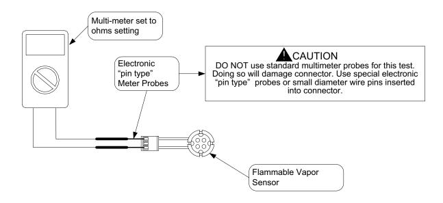
TTW SERVICE PROCEDURE VIII Safety Circuit Voltage Trace
