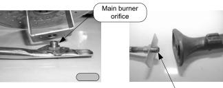
L.P. Main burner orifice. Left hand thread
