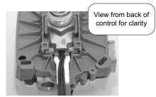
Step 5. Pivot tool towards heater as far as possible (see photo below). Lift straight up on gas control. The control should move about 1/8". At this point, remove tool not allowing the control to fall back. With tool removed, lift straight up on control to remove completely from Thermal Well.
