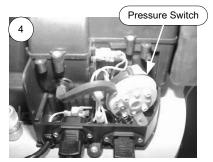
Slide pressure switch in direction of arrow while tilting slightly away from blower housing.
