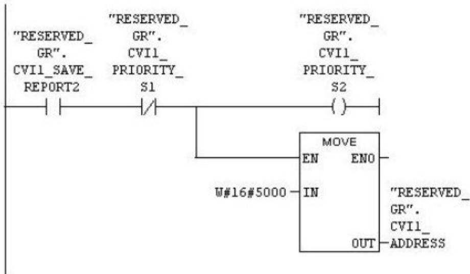
**Network 5 : END OF READING RESULT SPINDLE 1 (DONE) RESET THE SAVE BIT**
