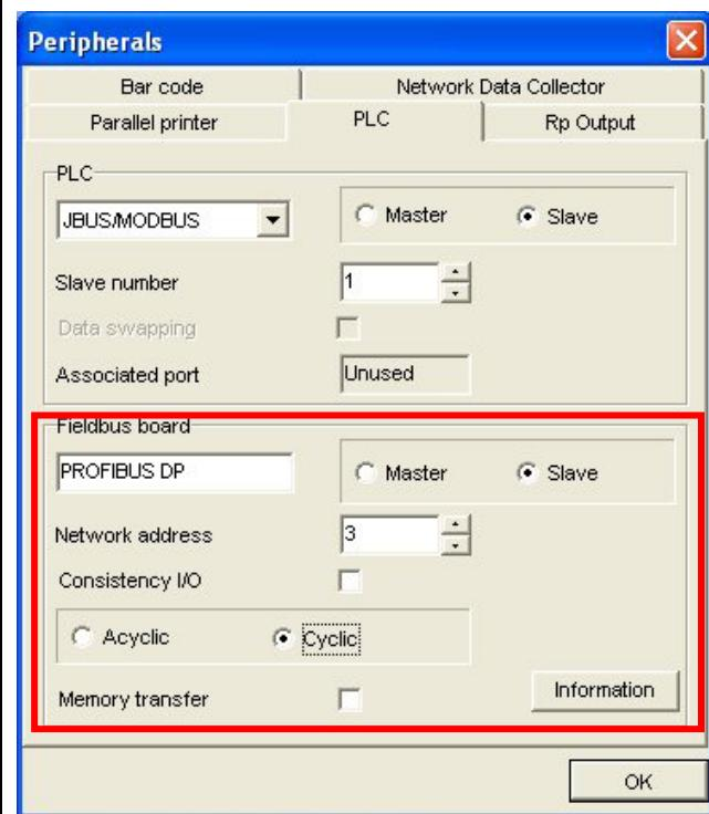
On the CVI: change and complete the ProfiBus DP address in accordance with the PLC configuration.
