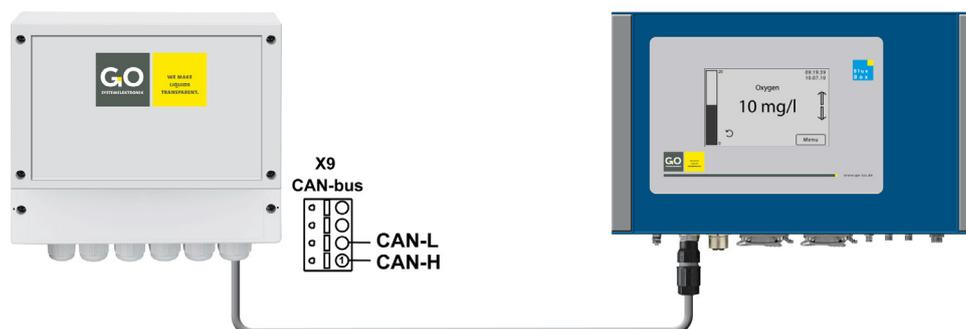
Connect the cable with CAN-H and CAN-L at the BlueSense Module (see connection diagram page 6 or 7). Connect the BlueBox with a fitting M12-connector.
