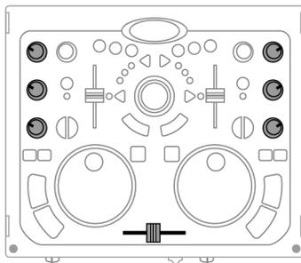
Switching from Deck A to Deck B (keep the cross fader in the center position for approximately 5 seconds while you adjust the Bass, Medium and Treble knobs on Deck A and Deck B).
